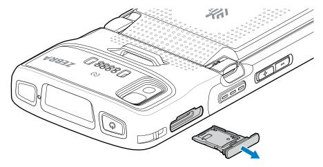
2. Place the microSD card, contact end first, with contacts facing up, into the card holder.
