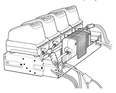
**11.** Secure the top tray to the bottom tray with four M5 screws (two on each side).
