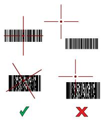
When the RS5100 is in Pick List mode, the RS5100 does not decode the barcode until the center of the crosshair touches the barcode.
