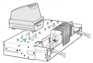
10. Connect DC Y cables to the four 4-Slot Battery Chargers.
