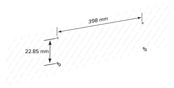
**3.** Align the mounting bracket's bottom mounting key holes with the screws.
