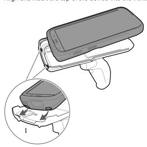
2. Rotate the device down and press down until it snaps into place.
