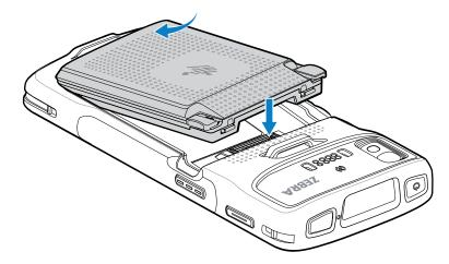
2. Press the battery down into the battery compartment until the battery release latches snap into place.
