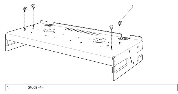
**7.** Align and install 5-Slot cradle onto studs of top tray.
