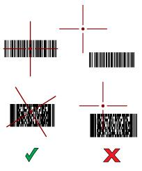
When the RS507/RS507X is in Pick List mode, the RS507/RS507X does not decode the barcode until the center of the crosshair touches the barcode.
