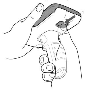
**2.** Lift the bottom of the device up and remove from the Trigger Handle.
