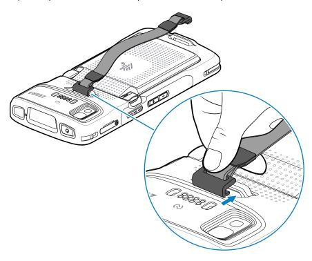
**2.** Clip the other end of the hand strap into the hand strap slot on the bottom of the device.
