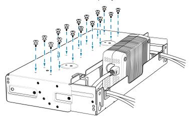
**9.** Align and install a 4-Slot Battery Charger onto each set of four studs.
