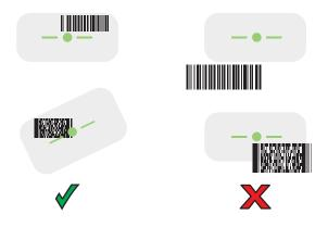
When the RS6100 is in Pick List mode, the RS6100 does not decode the barcode until the center of the crosshair touches the barcode.
