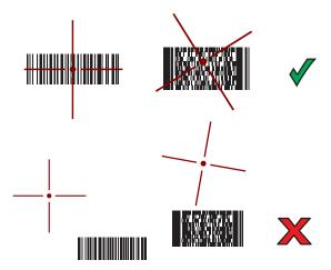
When the RS6000 is in Pick List mode, the RS6000 does not decode the barcode until the center of the crosshair touches the barcode.
