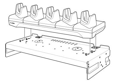
**8.** Secure cradle to top tray with two M2.5 safety screws.
