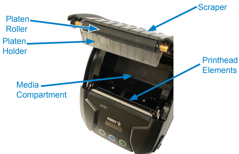
Figure 20 • Cleaning (Linerless)
